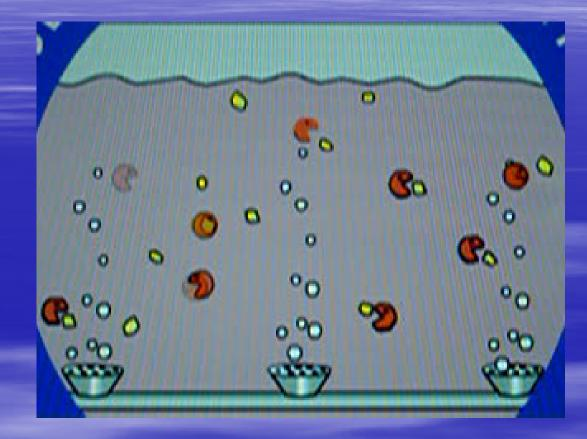
The circulating grit tank is a Vortex Grit Removal system. This type of system uses an adjustable mechanical grit tank circulator to set up a three dimensional flow pattern that gently rolls the basins contents and allows the heavier material to settle into the sump. Once the grit has been settled in the sump, it is removed by a grit pump which pumps the material to the main floor where it is dewatered using a static dewatering screen. The material is hauled to the landfill.
