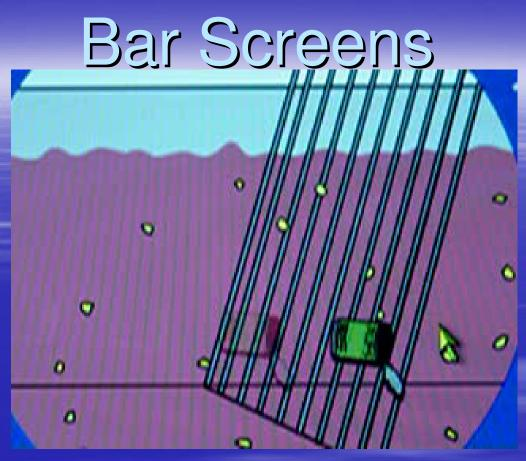
•A bar screen with evenly spaced vertical bars is placed at the beginning of a Wastewater Treatment Plant to remove large trash, sticks, plastic material, rags, ect. It is important to remove these materials because they could cause damage to equipment and decrease the capacity of the treatment plant. The captured material is then removed and properly disposed of.
