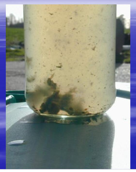
The anaerobic zone is the layer at the very bottom of the lagoon where no oxygen is present. This area includes a layer of sludge, which forms from the solids that settle out of the wastewater. Here, wastewater is treated by anaerobic bacteria, microscopic organisms, such as certain protozoa, and sludge worms, all of which thrive in anaerobic conditions.
